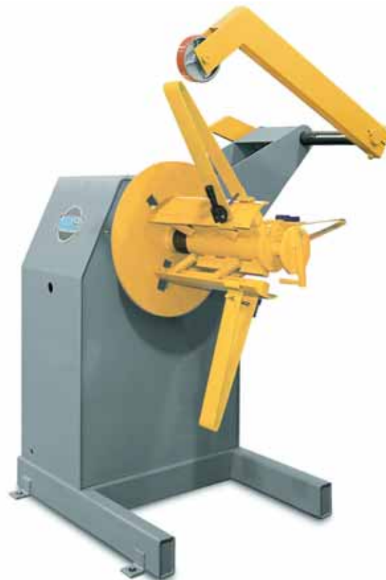
■ Standard 2,500# Series reel configured for "pull-off" application with manual hand crank expansion with a snapout handle, and a 30" diameter heavy duty backplate.
